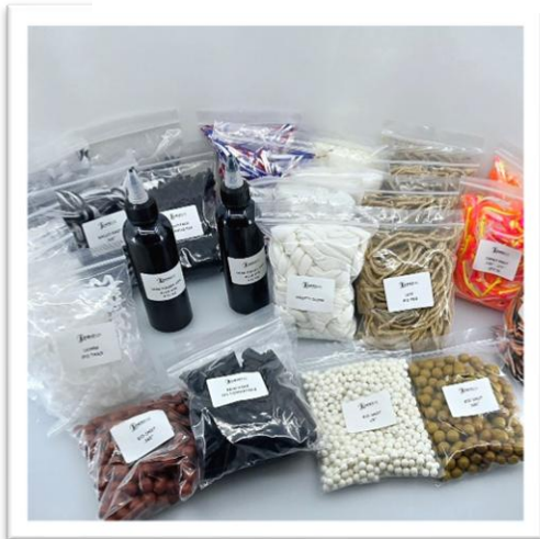
Figure 2- Junk Shot Kit Components
