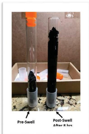
Figure 1- SwellFrac 400% Swell Out. All the samples shown were the same size
